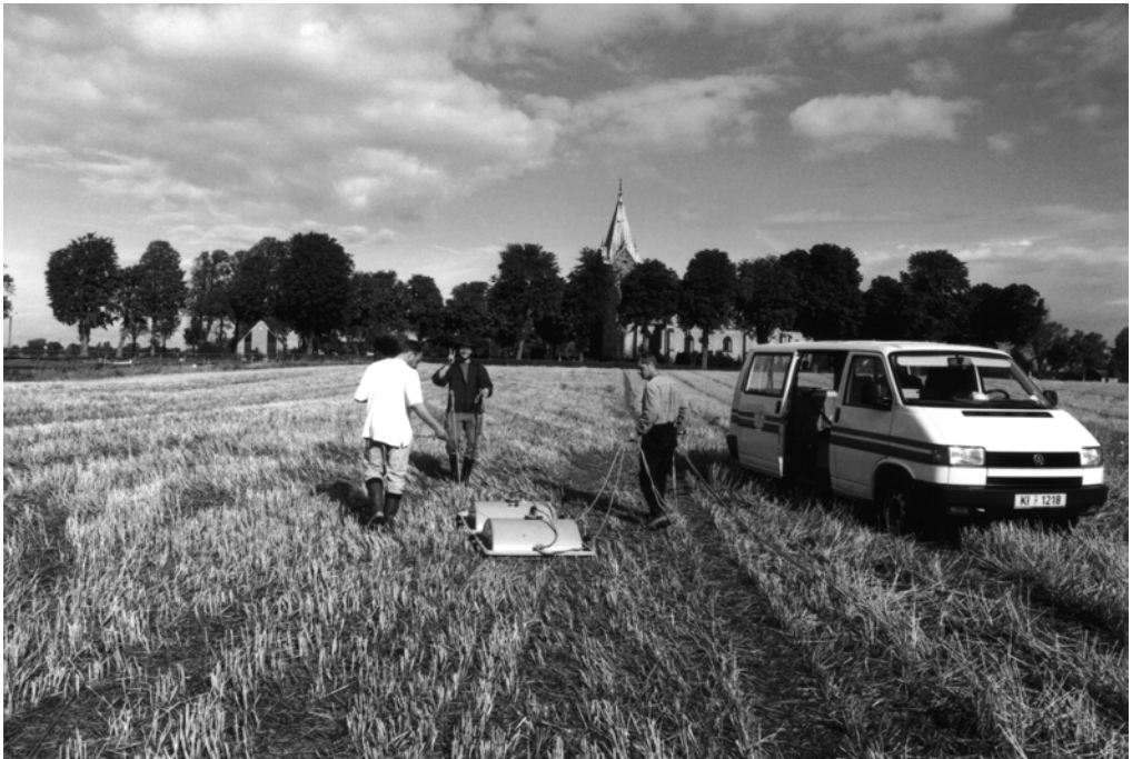
Fig. 2. GPR prospecting system using the 120 MHz antennas.
